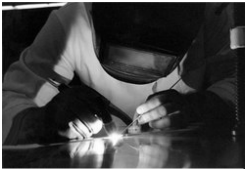
Gas tungsten arc welding
