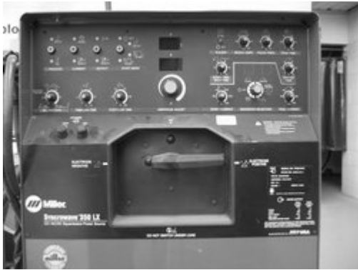
A constant current welding power supply capable of AC and DC
