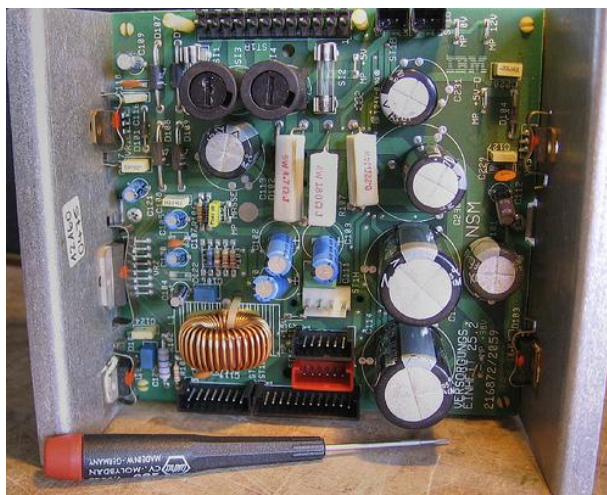
Figure 8: Example of a power supply. Image courtesy of markusram, Flickr.
